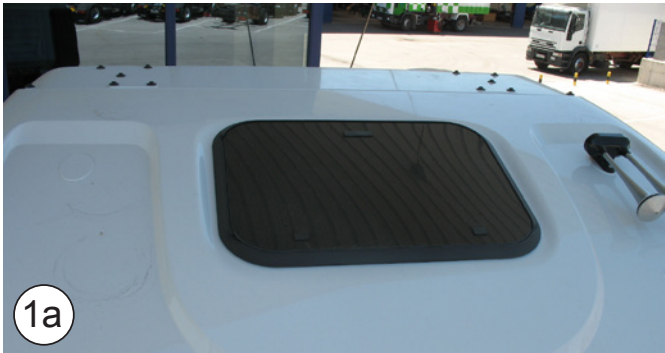
Stralis Cabin before 2008: 40 x 40 EPDM joint
